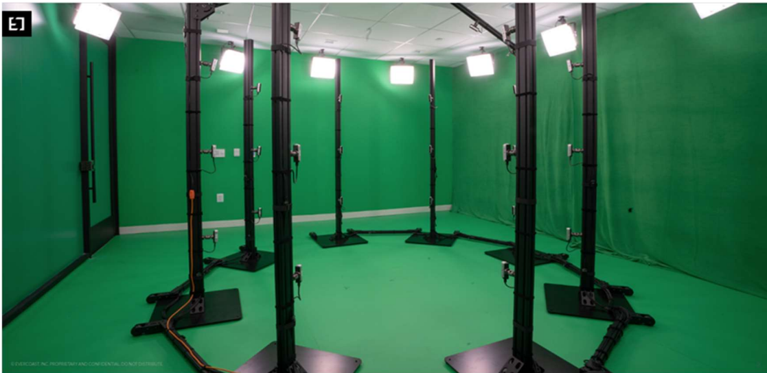
20 camera Evercoast Mavericks System deployed in a 12' x 12' conference room in Los Angeles, CA
